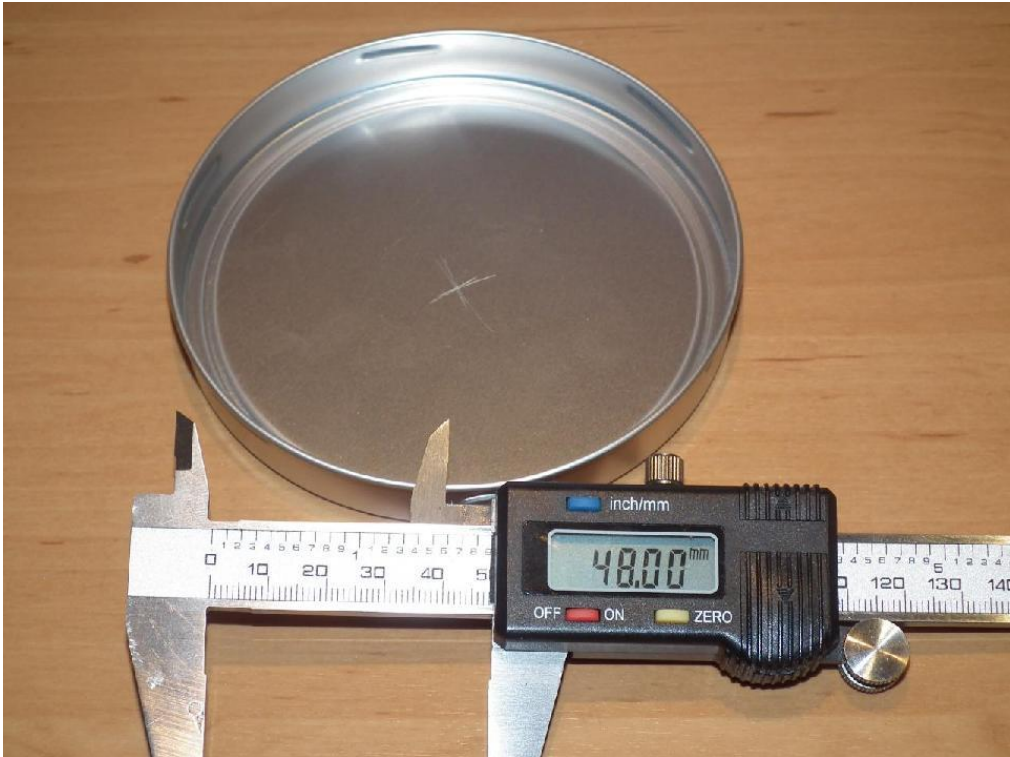
Step 45 - The centre of the cover is determined with a caliper. The radius to the groove is 48mm - The centre point is marked using the calipers of the gauge.
