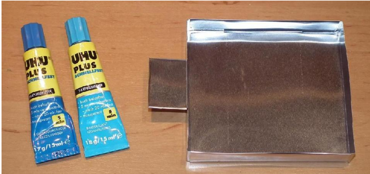
The completion of the firebox was surprisingly quick. A little 2C glue in the angle between the handle and the front side wall should prevent the sheet metal from tearing during frequent use.
