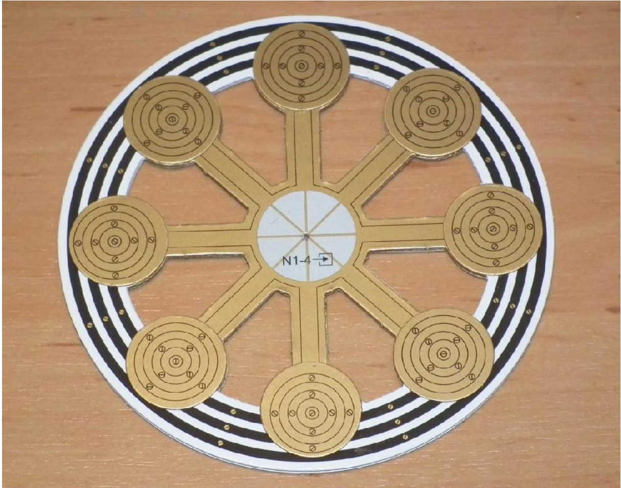
The finished flywheel after colouring the edges with gold and white paint.
