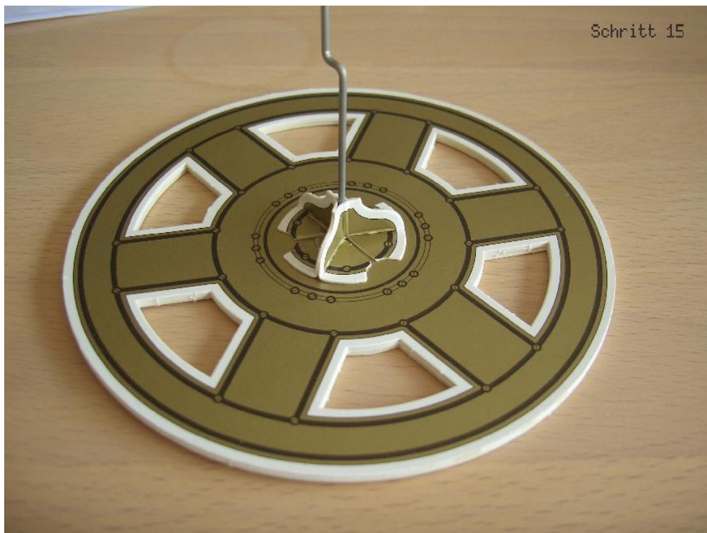
Step 15: Flywheel with axle and its holder.
