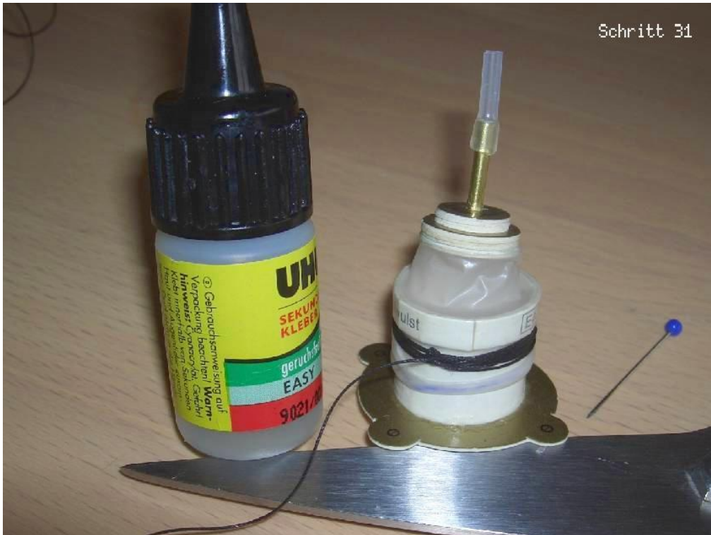
Step 31: Fixing the seal to the working cylinder, the knot of the yarn was fixed with superglue.
