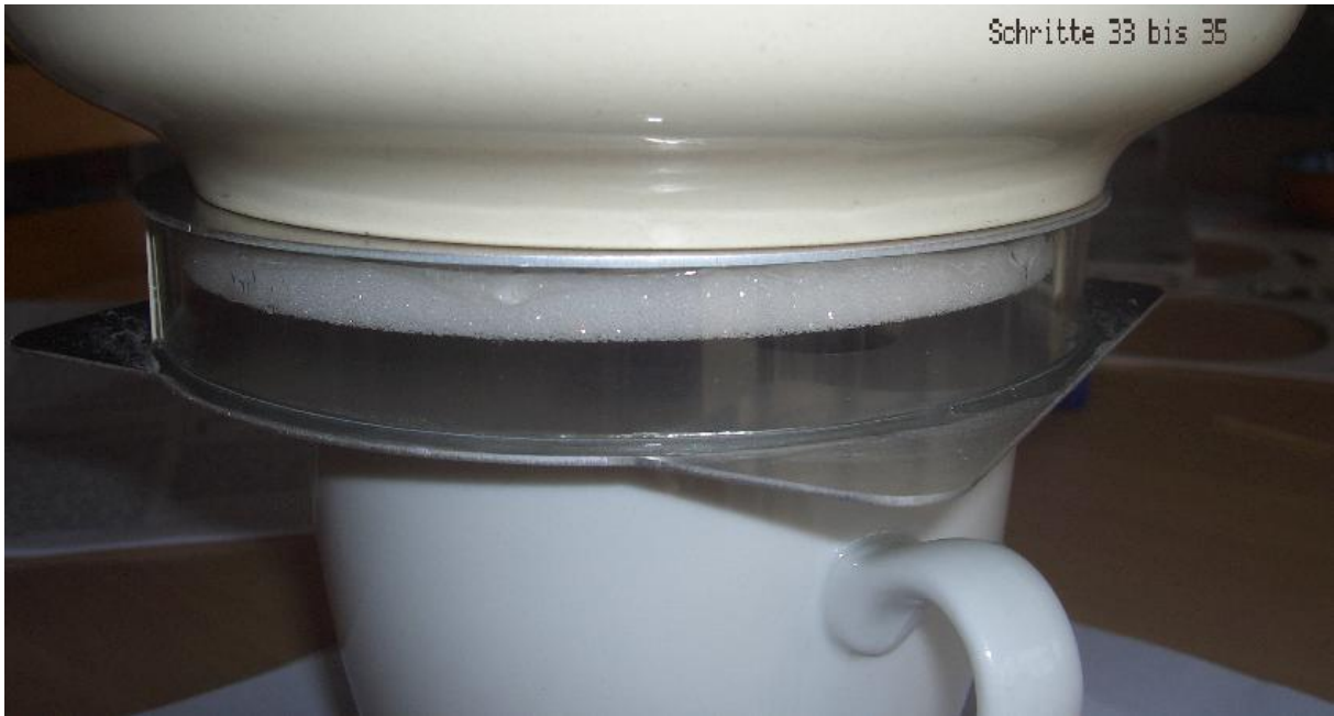
Steps 33 – 35: Gluing the cylinder cover to the cylinder wall.
