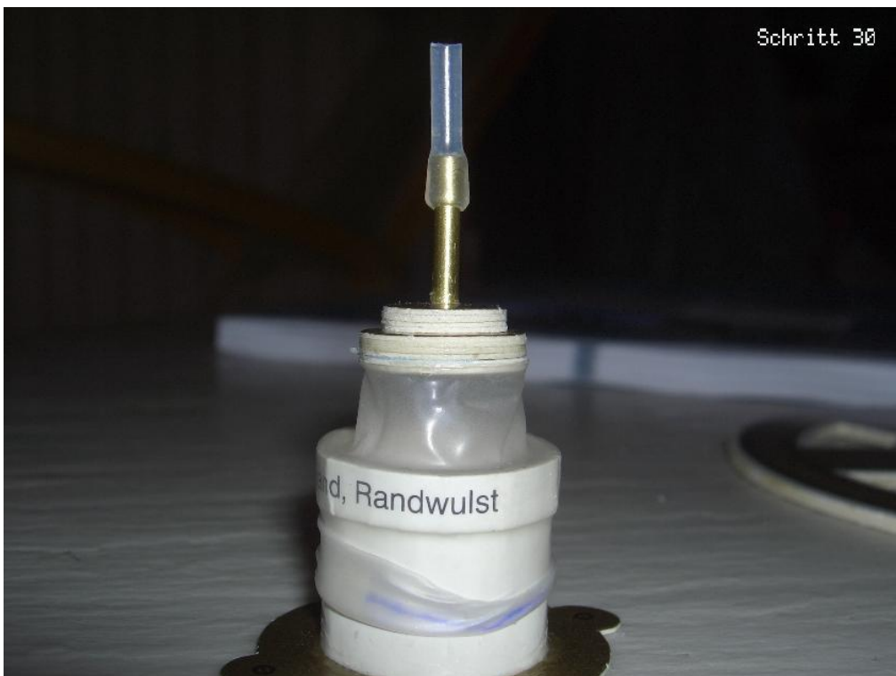
Step 30: Connection of working cylinder and piston.
