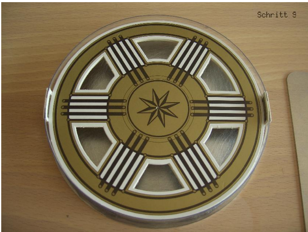
Step 9: ...glue the wall to the base plate using the flywheel as a centring device.
