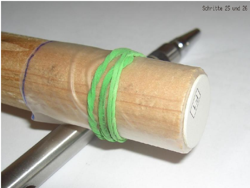
Steps 25 & 26: Pointer finger of a vinyl glove as a seal, cardboard disc glued to it as the base plate of the working piston.
