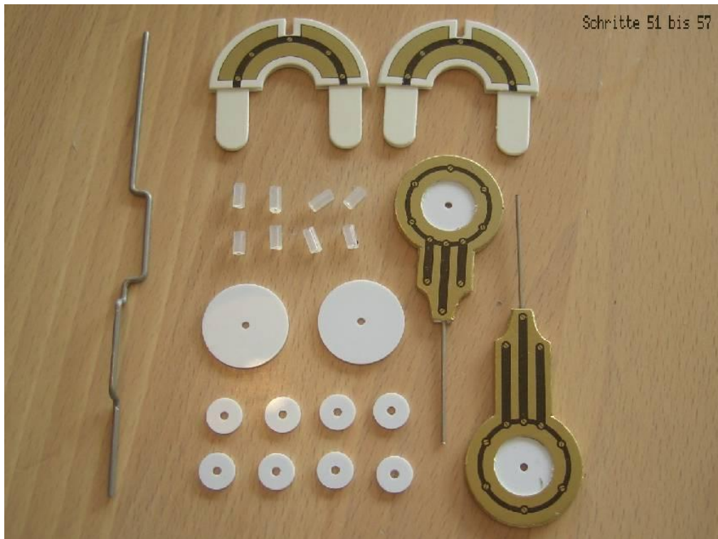
Steps 51 – 57: The parts needed to assemble the crankshaft.
