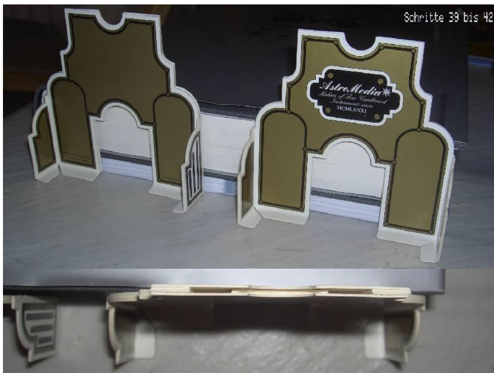
Steps 39 – 42: Stand with angled supports and view into the mounting holes for the bearing holders.
