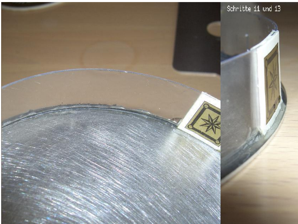
Steps 11 & 13: Wall of the master cylinder bonded to the base plate.
