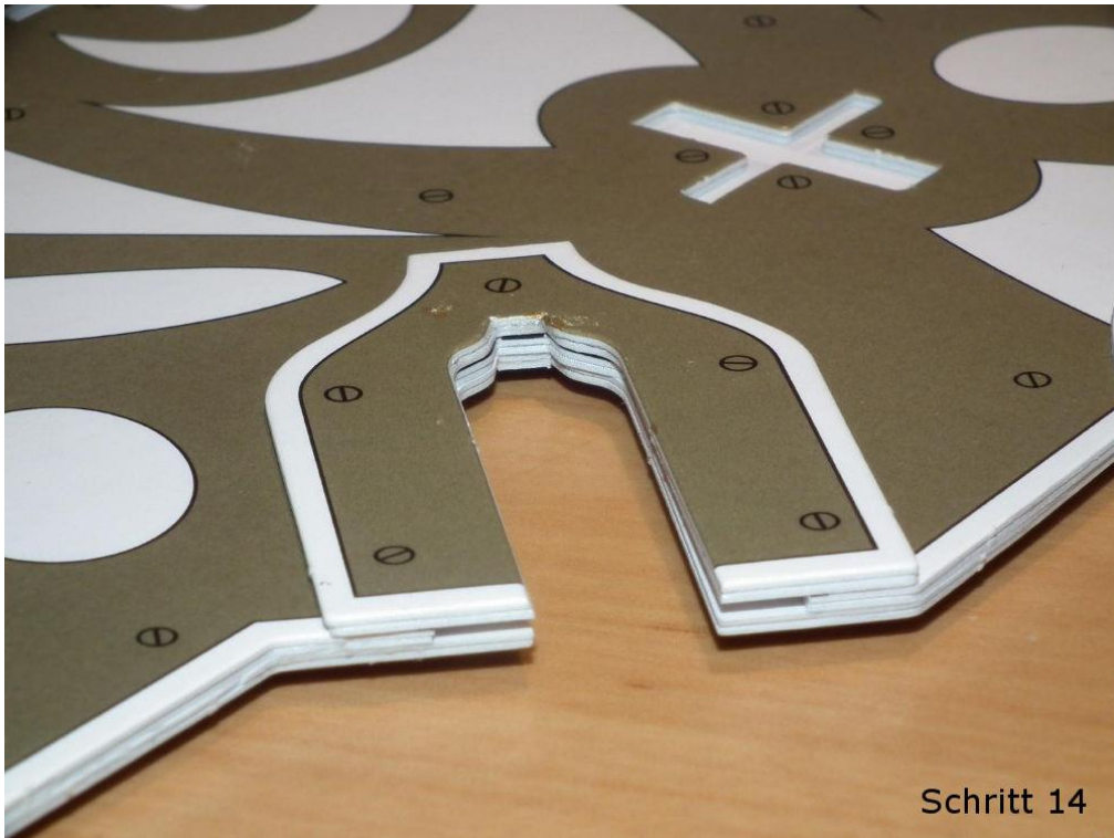
Step 14: Ready mounted guide of the sun filter slide.
