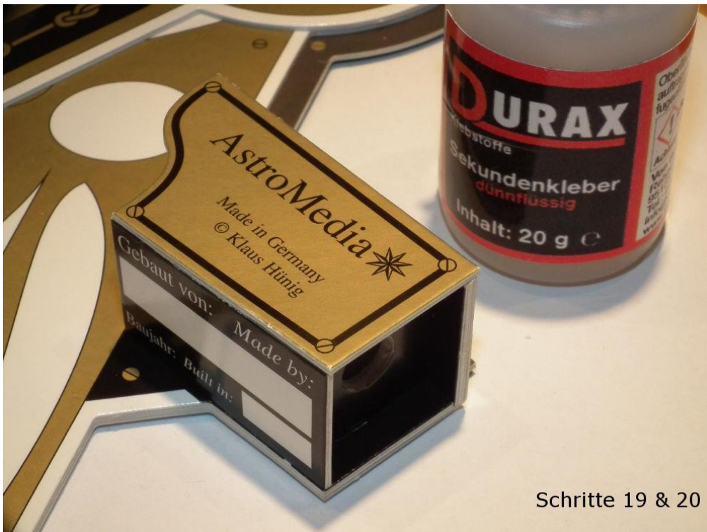
Steps 19 & 20: The finished bearing housing after mounting the base and the side cover. The housing was glued together with superglue to shorten the drying time. If you want to handwrite your name and the year of manufacture, you should do this before mounting the housing. Alternatively, printed stickers can be applied later (see step 38 below).
