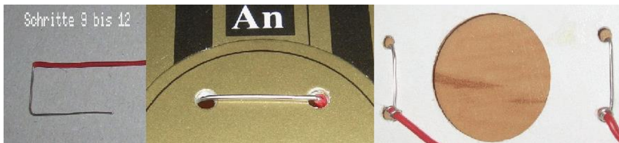
Steps 9 – 12: Attachment of the contacts on the lamp and battery side of the switch in the housing.
