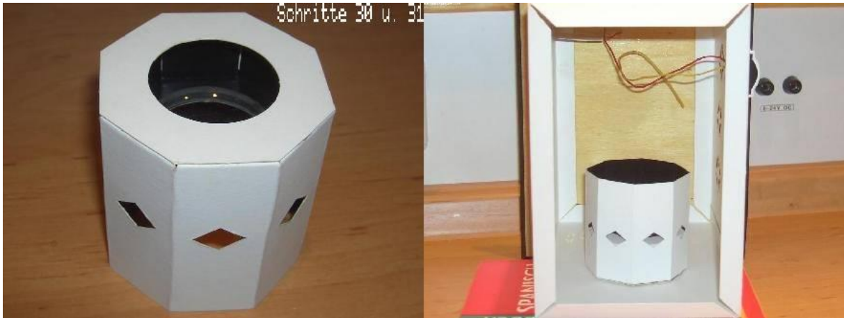
Steps 30 & 31: The creation of the condenser (2) and its installation in the housing.
