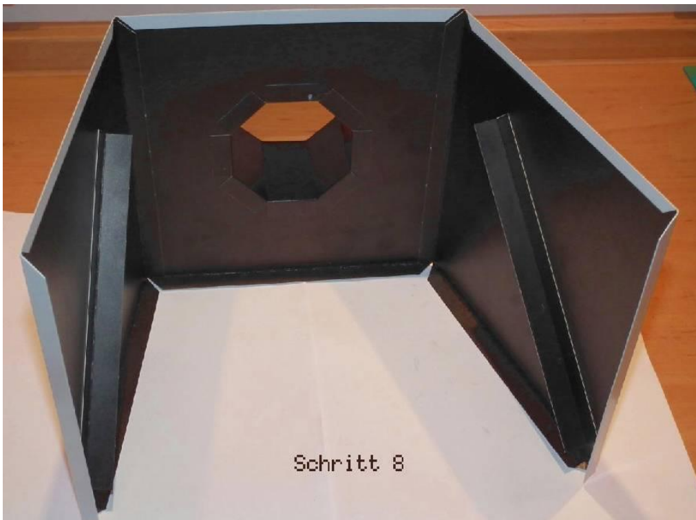
Step 8: The paper strips glued to the inside of the side walls, serve as mirror holders.
